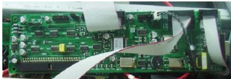
Figure4.3.1.1 The Control board.
