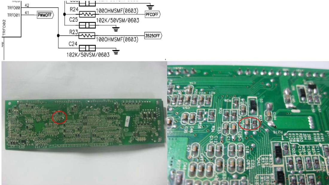
2. Check the components D13,D14,D15 connected TX1 not damaged, be sure the TX is not broken
