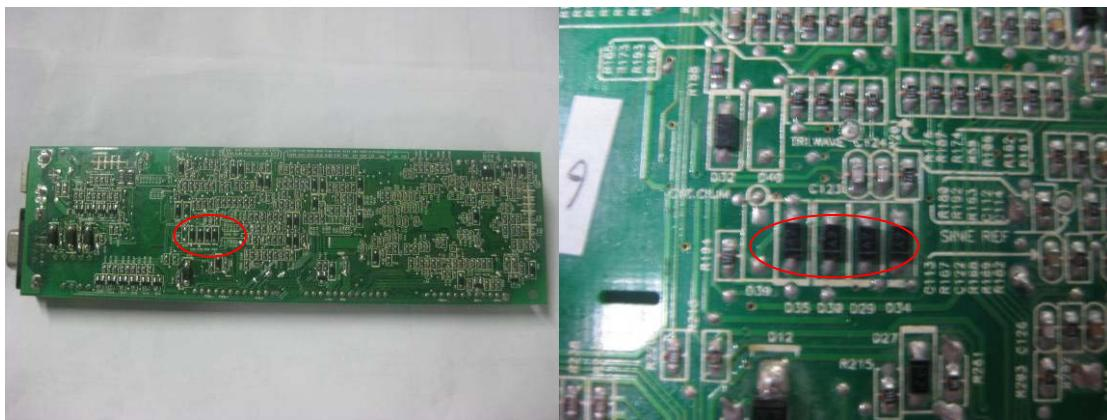
3. Check the U110 pin 5 whether shorted to ground, if shorted replace U110: IC2003
