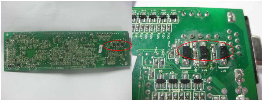
3. Check the U107 surrounding components, R257, C138 ,D23,C108,D38,C136,if these all ok , maybe you need to replace the U107: TL074 , at last , maybe the MCU is broken.
