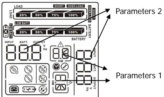
Two parameters need to be configured in order to set up the UPS. Refer to following diagram.
