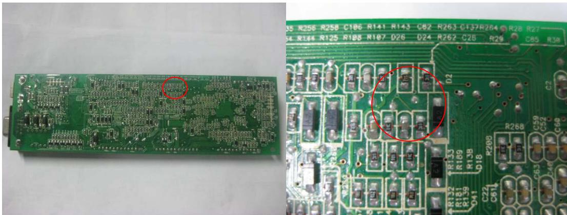
2. no LCD display , but DC fans operate , maybe the MCU broken
