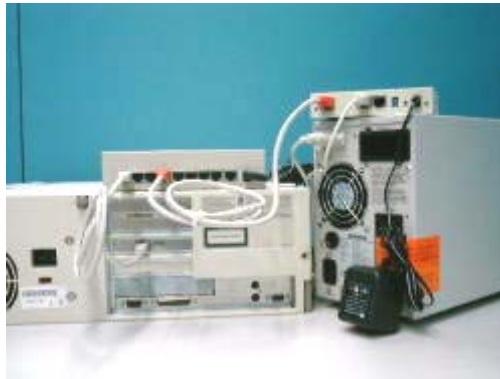
Figure 9 Connecting the Ethernet cable from the LAN port of WEBPOWER/Mate.
