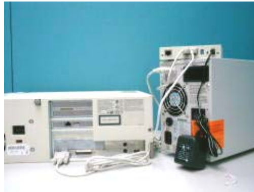
Figure 2-4 Serial cable connection of WEBPOWER/Mate
