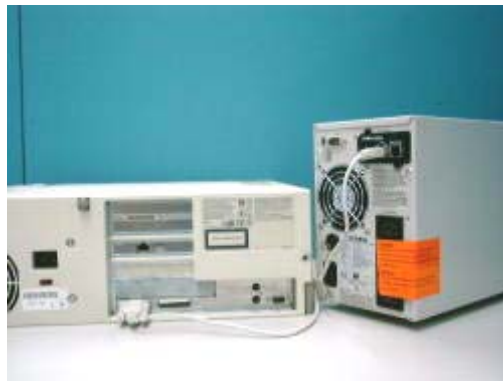
Figure 2-3 Serial cable connection of WEBPOWER Plus/WEBPOWER Pro
